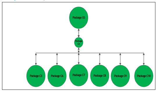
Figure 4-4. Package C-State Entry and Exit
