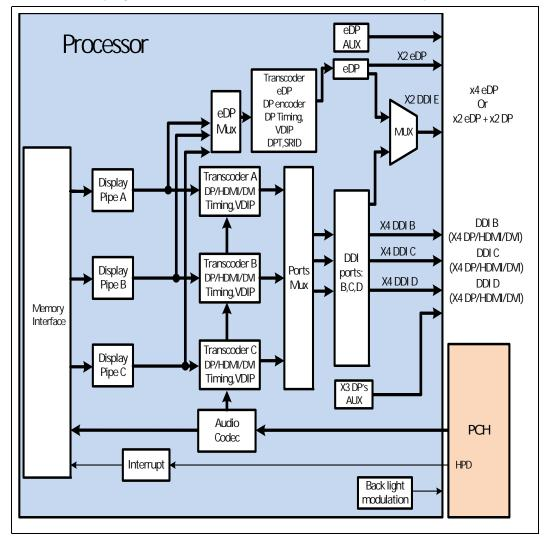
Figure 2-5. Processor Display Architecture (with 3 DDI Ports as an Example)
