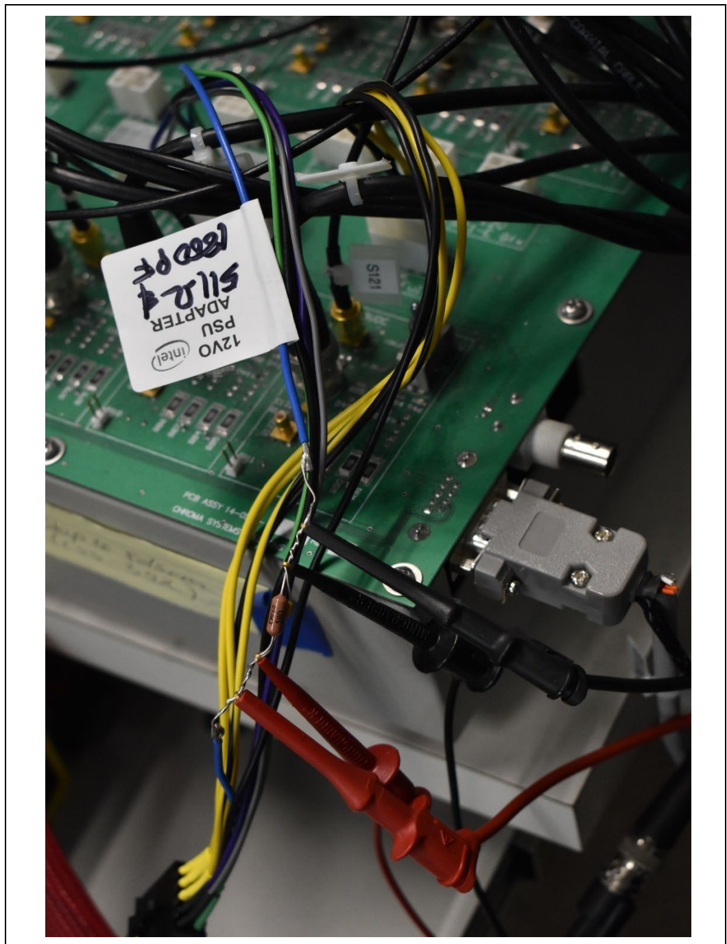
Figure 6-1: Test Fixture Example Measurement Location for I_PSU% Signal
