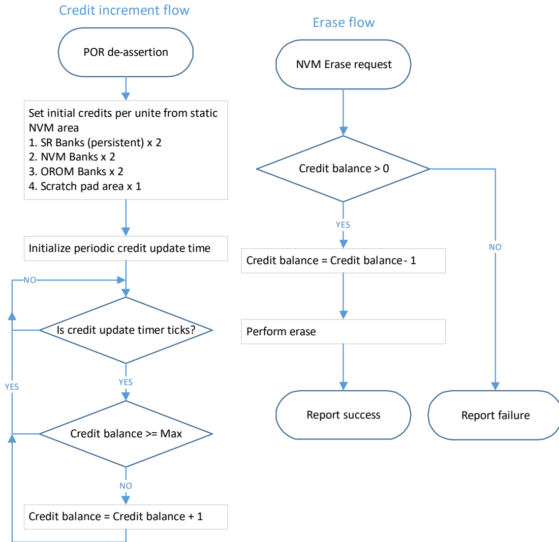
Figure 3-33. Flash Wear-Out Protection Algorithm 1
