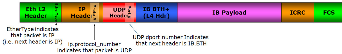
Figure A-41. RoCEv2 Packet Format
