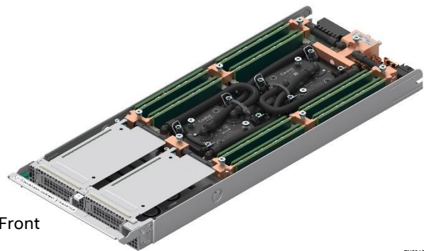
1U Liquid-Cooled Compute Module
