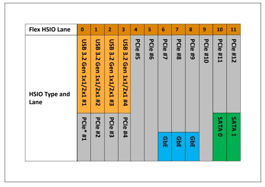
The 12 Flexible HSIO Lanes [11:0] on PCH-LP (UP3) support the following configurations:
