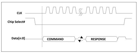
An eSPI transaction consists of a Command phase driven by the master, a turn-around phase (TAR), and a Response phase driven by the slave.
