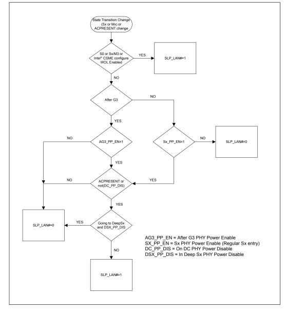
Figure 14. Conceptual Diagram of SLP\_LAN#
