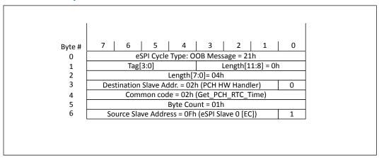
Figure 9. **PCH Response to eSPI Slave with RTC Time**
