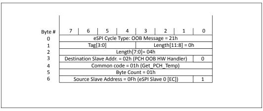
Figure 7. PCH Response to eSPI Slave with PCH Temperature
