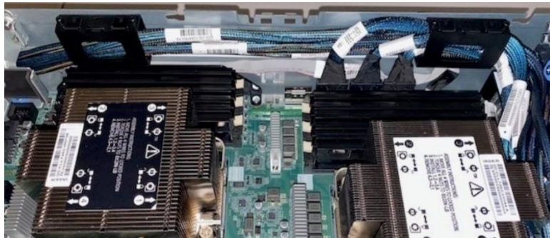
Figure 17. Internal Cable Management
