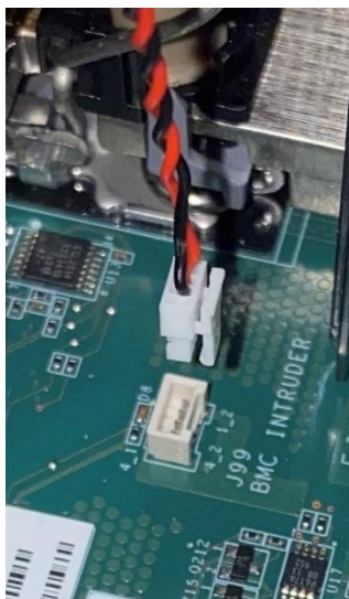
Figure 12. Chassis Intrusion Switch Cable to Server Board
