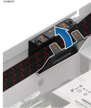
Cables routed and secured
