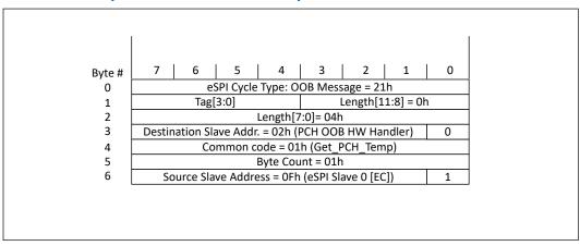
Figure 6. PCH Response to eSPI Slave with PCH Temperature
