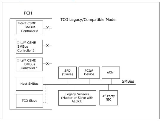
In TCO Legacy/Compatible mode the PCH can function directly with an external LAN controller or equivalent external LAN controller to report messages to a network management console without the aid of the system processor. This is crucial in cases
