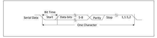
The UART Host Controller Line Control Register (LCR) is used to control the serial character characteristics. The individual bits of the data word are sent after the Start bit, starting with the least significant bit (LSB). These are followed by the optional parity bit, followed by the Stop bit(s), which can be 1, 1.5, or 2.
