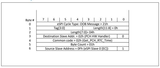
Figure 8. PCH Response to eSPI Slave with RTC Time
