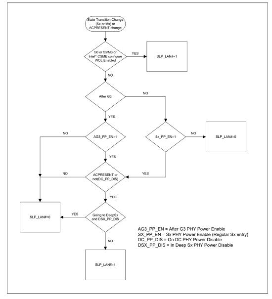
Figure 13. Conceptual Diagram of SLP\_LAN#
