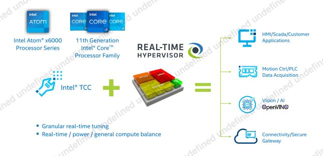
Attaining virtualized real-time requirements by enabling workload consolidation of real-time and non-real-time workloads.
