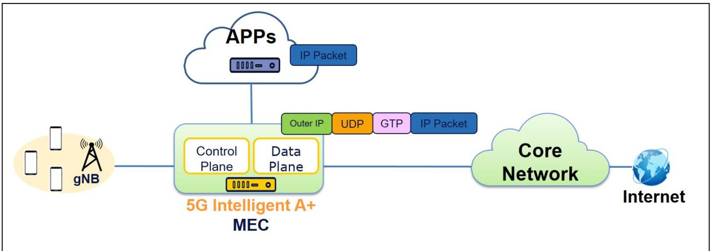
Figure 2. Components of Chunghwa Telecom\* 5G Intelligent A+
