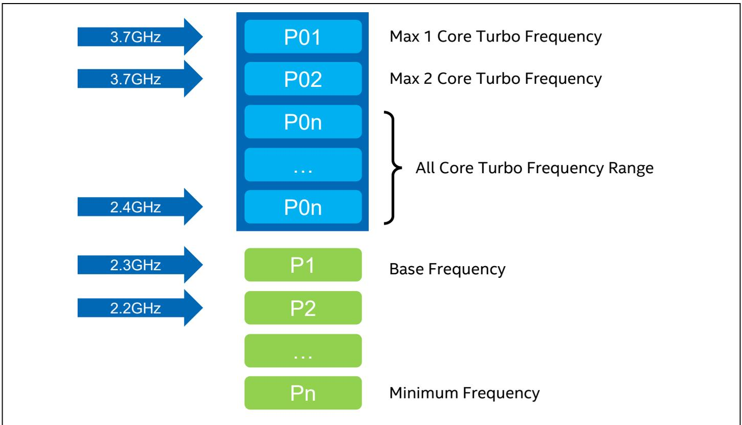
Figure 4. Intel® Xeon® Silver 5218N: Non-Intel® AVX Intel® Turbo Boost Technology 2.0 Frequency
