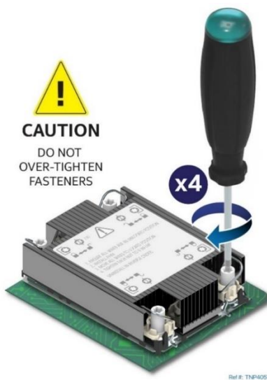
Figure 144. Tighten Heat Sink Fasteners
