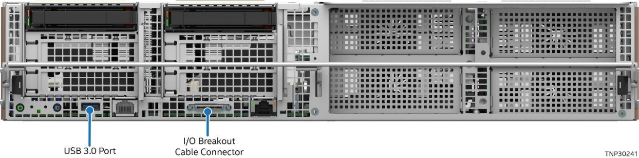
Figure 83. USB Port Location - 2U Accelerator Module
