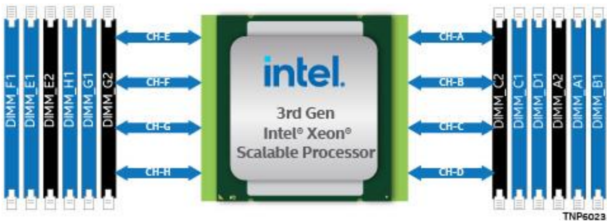
Figure 55. Memory Slot Connectivity for D50TNP1SB
