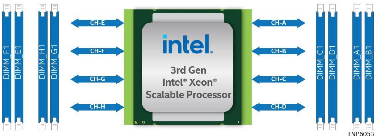
Figure 56. Memory Slot Connectivity for D50TNP1SBCR
