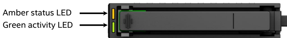
Figure 68. Drive Carrier LED Identification
