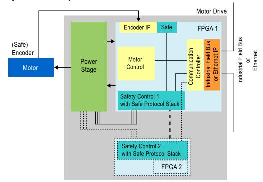
Figure 6. Dual-FPGA Implementation for a Safe Drive
