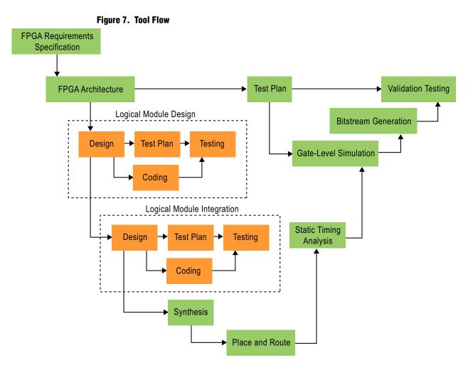
The V-Flow and the documentation that comes along with it maps all steps in the design of a safe application for Altera FPGAs to the IEC specification and its requirements. In addition, it explains which Altera tools are used for the specified design steps. Specific chapters in the IEC specification are discussed and an explanation is provided to guide the Altera user to follow the right development steps for the development of a safe application.
