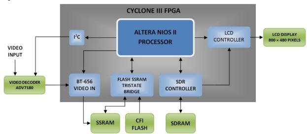
Figure 5. Internal Architecture
