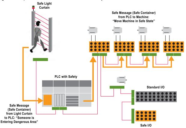
Figure 2. Complex Fieldbus-Networked Coordinated Safety Machine
