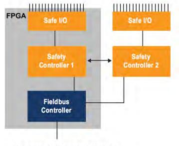
Figure 6. Flexible Altera FPGA Simplifies Functional Safety Design
