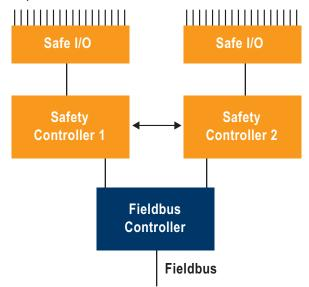
Figure 4. Typical Discrete SIL3 Implementation with Three Microcontrollers
