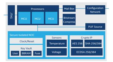
Figure 1. Secure Device Manager Functional Blocks
