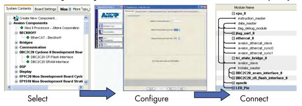
Figure 4. Using Hardware IP with SOPC Builder to Create an Industrial Ethernet-Capable System
