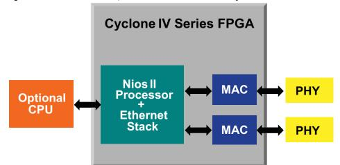
Figure 1. Generic FPGA-Based, 2-Channel Industrial Ethernet System
