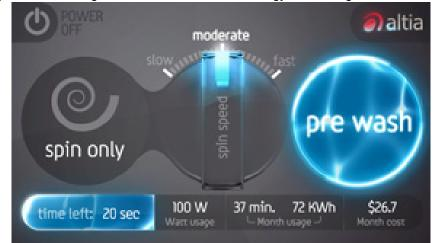
Figure 1. Example of a Washing Machine HMI With New Energy Monitoring Features
