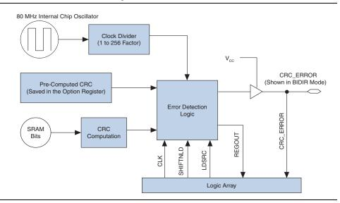
The user logic is affected by the soft error failure, so reading out the 32-bit CRC signature through the regout should not be relied upon to detect a soft error. You should rely on the CRC\_ERROR output signal itself, because this CRC\_ERROR output signal cannot be affected by a soft error.
