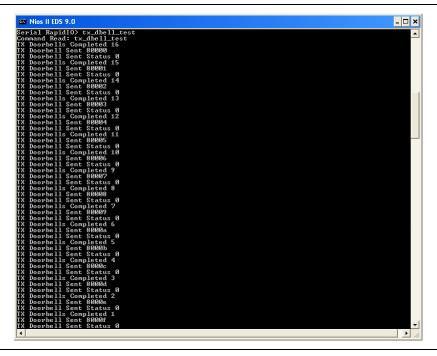
The TI DSP is programmed to handle only 64 outstanding messages. Therefore, the fifth group of Doorbell messages times out. The Doorbell Sent Status of each Doorbell message in the group indicates the timeout. Figure 21 shows the test output with Doorbell Sent Status indicating a timeout for each message in the fifth group of Doorbell messages sent from the RapidIO MegaCore function in the FPGA.
