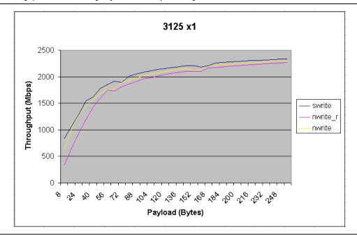
Figure 28. Throughput with Increasing Payload in ×1 RapidIO MegaCore function at 3.125 Gbaud
