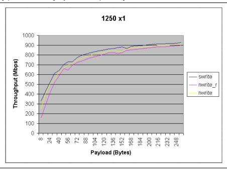
Figure 27. Throughput with Increasing Payload in ×1 RapidIO MegaCore function at 2.500 Gbaud
