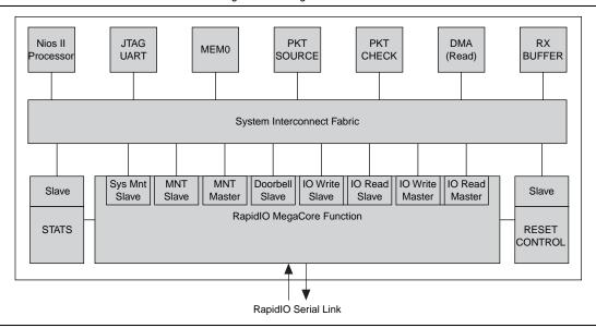
The pkt\_source and pkt\_check components appear in the packet-generator based design but not in the DMA-based design. All other system components function identically in the DMA-based and packet-generator based versions of the design.
