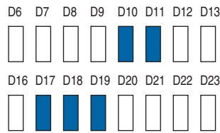
Figure 5. Condition of LEDs for Parallel Loopback Demonstration
