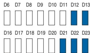
Figure 7. Condition of LEDs for Receiver Demonstration
