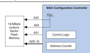
Figure 8. 8-Bit Wide, 16-MByte Uniform Sector Flash Connection
