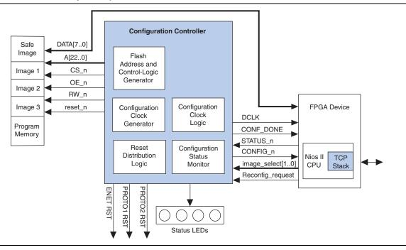
The Nios Embedded Evaluation Kit, Cyclone III Edition and the Altera Embedded Systems Development Kit, Cyclone III Edition include an application selector utility as their factory design. The application selector utility is capable of remote update using Ethernet.
