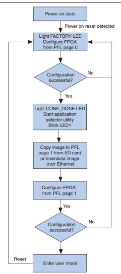
Figure 7. Altera Embedded Systems Development Kit, Cyclone III Edition Configuration Controller Boot Sequence Flowchart
