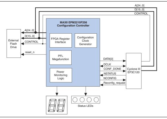
Figure 6. Development Board Configuration Controller for the Altera Embedded Systems Development Kit, Cyclone III Edition
