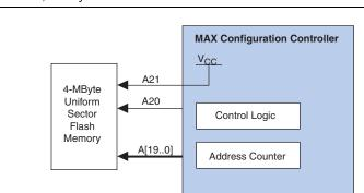
Figure 9. 8-Bit Wide, 4-MByte Uniform Sector Flash Connection
