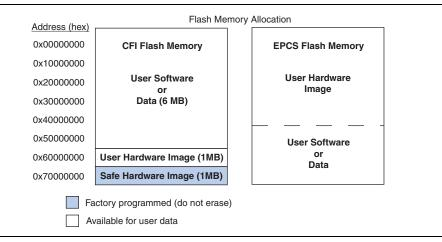
The first section is used for general programming or data storage. The other two sections—user and safe image—store FPGA hardware configurations. The user image typically contains a hardware design that is under development or testing. The safe (factory programmed) image typically contains a working, default hardware image.
