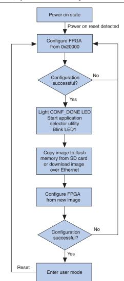
Figure 5. Nios II Embedded Evaluation Kit, Cyclone III Edition Configuration Controller Boot Sequence Flowchart
