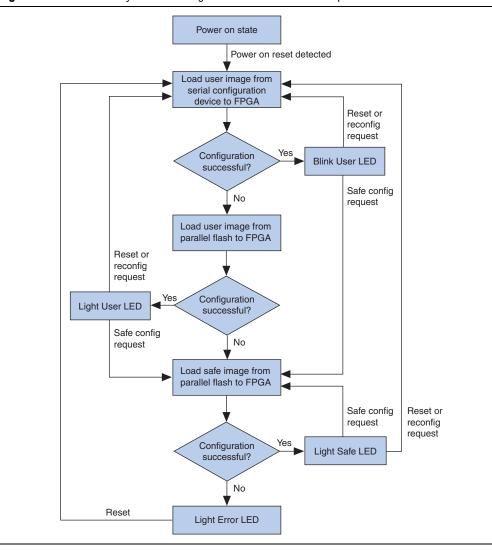
Figure 2. Stratix II and Cyclone II Configuration Controller Boot Sequence Flowchart
