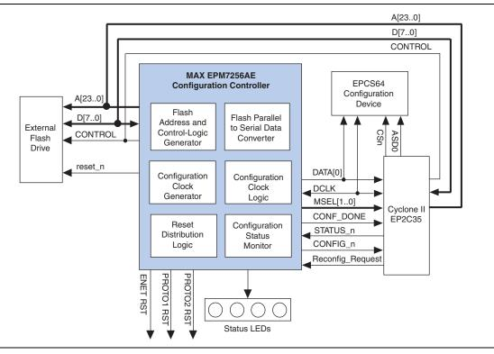
The main differences between the Cyclone II edition and Stratix II edition development board's configuration controllers are that the Cyclone II edition includes a parallel to serial converter block and control logic block modifications. The parallel to serial block reads an 8-bit word from the flash image every 8 DCLK cycles and shifts the word out to the DATA0 input of the Cyclone II device on every DCLK cycle.
