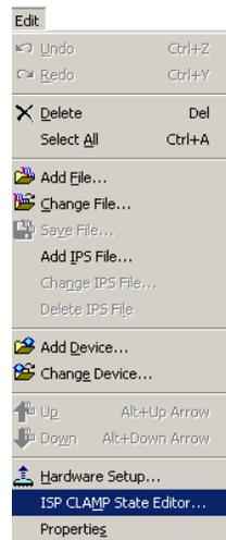
4. Specify the states of the pins in your design in the ISP Clamp State Editor. There are four clamp state choices: tri-state, high, low, and sample and sustain. By default, all pins are set to tri-state.
