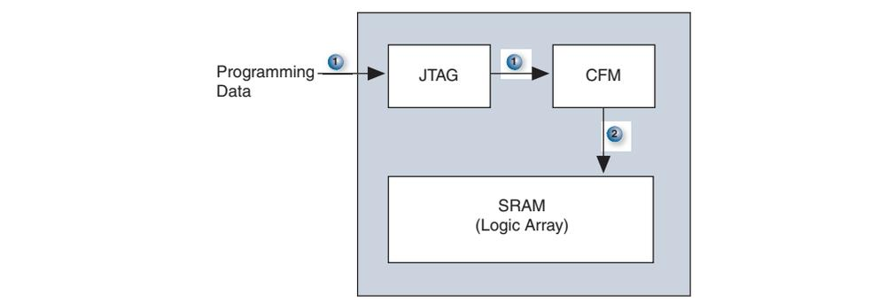
In real-time ISP mode, the user flash memory (UFM), programmable logic, and I/O pins remain operational while programming of the CFM is in progress. The contents of the CFM will not download into the SRAM after the successful programming of the CFM. Instead, the device waits for a power cycle to occur. The normal power-up sequence occurs (CFM downloads to SRAM at power-up) and the device enters user mode after  $t_{\text{CONFIG}}$  time. Figure 12-2 shows the flow of real-time ISP.
