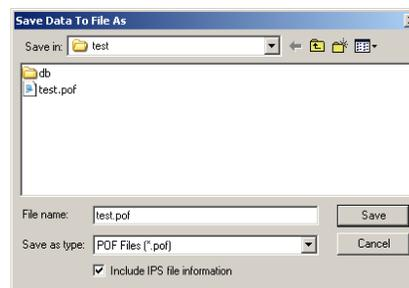
When programming a device with the ISP Clamp box checked, the Quartus II Programmer will first look for the IPS file. If the IPS file is not found, only then it will look into the POF for the pin state information.
