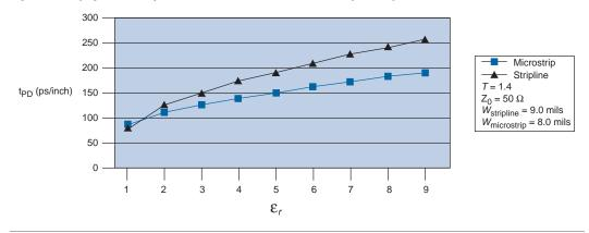
Figure 9. Propagation Delay vs. Dielectric Constant for Microstrip & Stripline Traces
