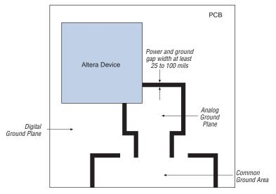
If your system shares the same plane between analog and digital power supplies, there may be unwanted interaction between the two circuit types. The following suggestions will help to reduce noise:
