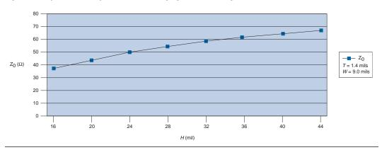
Figure 7. Stripline Trace Impedance with Changing Dielectric Height
