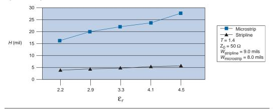
Figure 13. Height vs. Dielectric Constant
