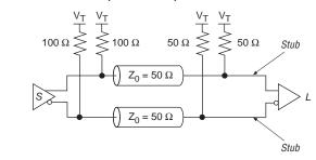
Figure 34 shows the differential pair, fly-by termination scheme for 3.3-V PCML.
