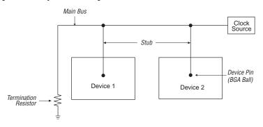
Figures 15 through 17 show the SPICE simulation with different stub length. As the stub length decreases, there is less reflection noise, and the eye opening increases due to less reflection noise.
