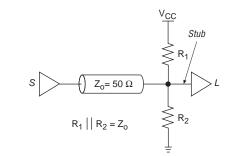
As noted in the previous section, stub length is dependent on signal rise and fall time and should be kept to a minimum. If your design requires a long termination line between the terminator and receiver, use fly-by termination or Thevenin fly-by termination. See Figures 23 and 25.
