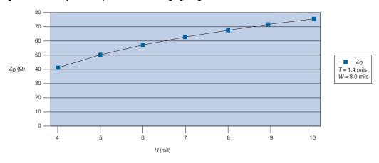
Figure 4. Microstrip Trace Impedance with Changing Height
