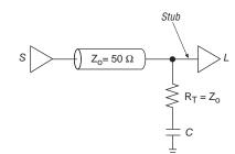
Figure 29 shows series-RC parallel fly-by termination.
