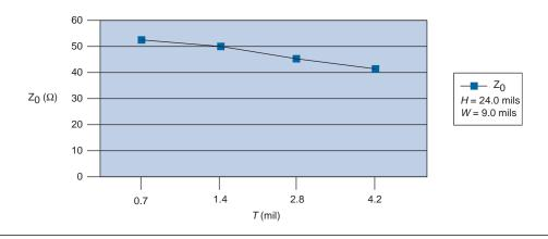
Figure 8. Stripline Trace Impedance with Changing Trace Thickness
