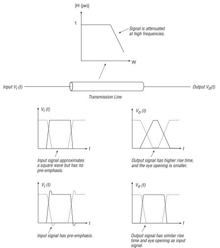
Stratix<sup>TM</sup> GX devices provide programmable pre-emphasis to compensate for variable lengths of transmission media. You can set the pre-emphasis to be between 5% and 25%, depending on the value of the output differential voltage (V<sub>OD</sub>). Table 2 shows the available Stratix GX programmable pre-emphasis settings.
