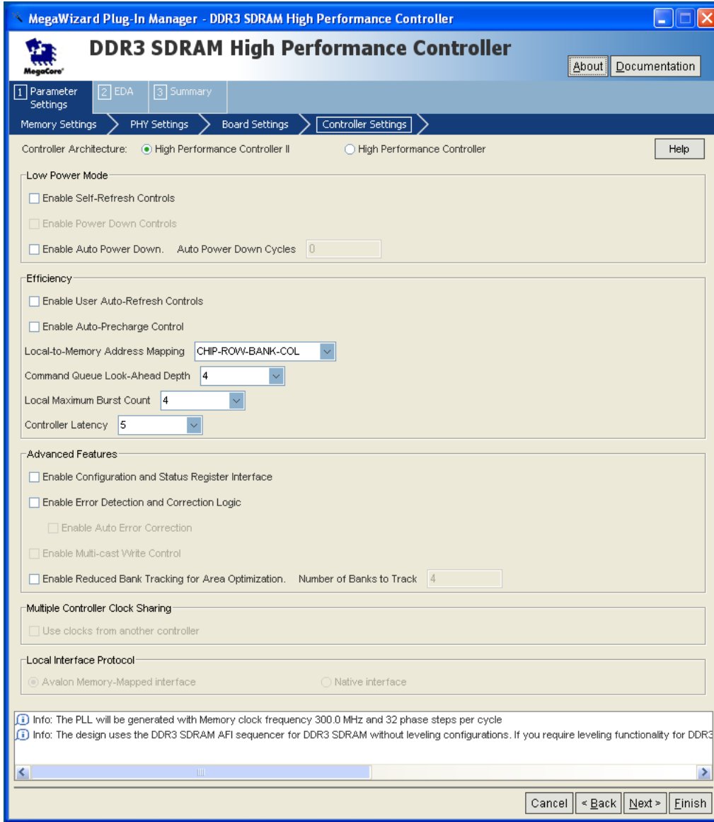
Figure 3-3. DDR3 SDRAM Controller with ALTMEMPHY Settings
