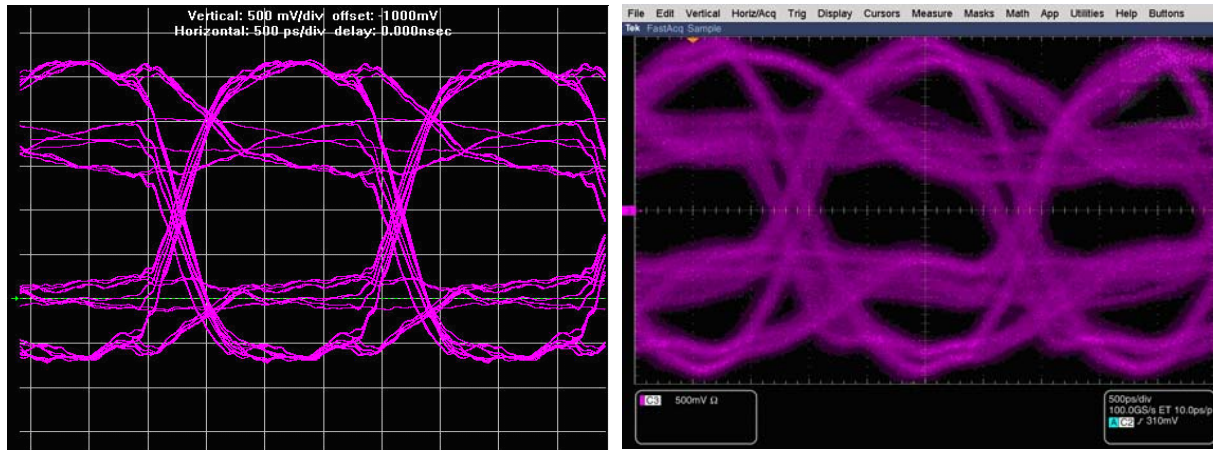
Figure 4–30. HyperLynx Simulation and Board Measurement, FPGA Writing to Memory
