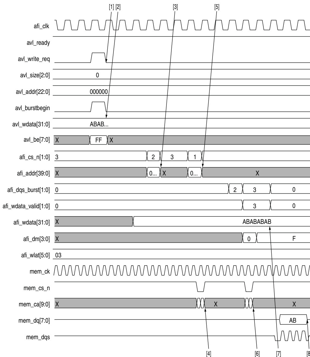
Figure 12-18. Half-Rate LPDDR2 Write
