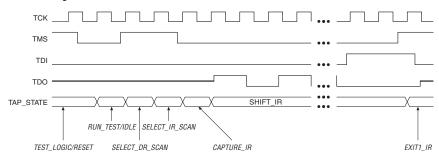
The TDO pin is tri-stated in all states except in the SHIFT\_IR and SHIFT\_DR states. The TDO pin is activated at the first falling edge of TCK after entering either of the shift states and is tri-stated at the first falling edge of TCK after leaving either of the shift states.
