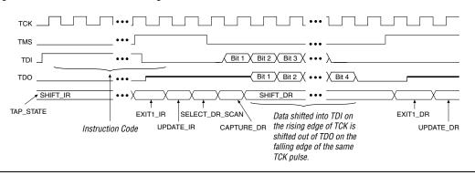
Figure 13–12. BYPASS Shift Data Register Waveforms
