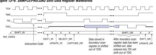
Figure 13–9. SAMPLE/PRELOAD Shift Data Register Waveforms
