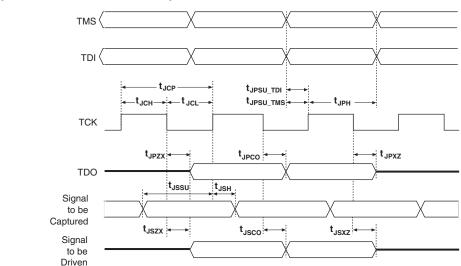
Figure 13-6. IEEE Std. 1149.1 Timing Waveforms
