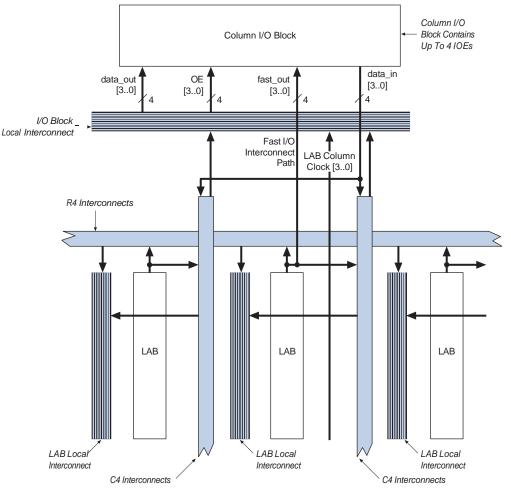
Figure 2–21 shows how a column I/O block connects to the logic array.
