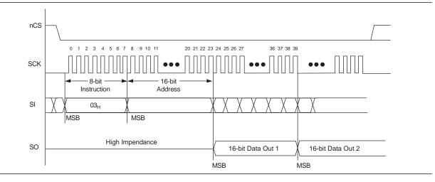
Figure 9–27 shows the READ operation sequence for Base mode.
