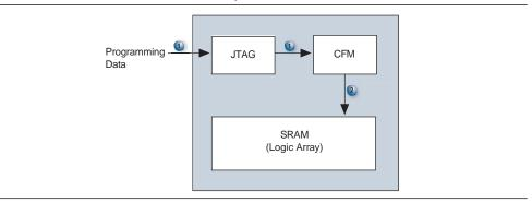
In real-time ISP mode, the user flash memory (UFM), programmable logic, and I/O pins remain operational while programming of the CFM is in progress. The contents of the CFM will not download into the SRAM after the successful programming of the CFM. Instead, the device waits for a power cycle to occur. The normal power-up sequence occurs (CFM downloads to SRAM at power-up) and the device enters user mode after  $t_{\text{CONFIG}}$  time. Figure 12–2 shows the flow of real-time ISP.
