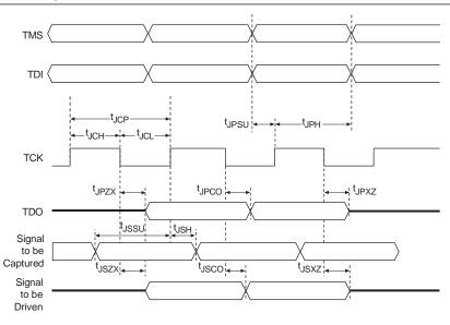
Table 5-34 shows the JTAG Timing parameters and values for MAX II devices.
