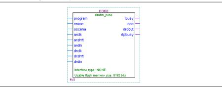
Figure 9-43. altufm Megafunction Symbol for None Instantiation
