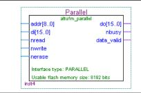
Figure 9–42 shows page 3 of the altufm MegaWizard Plug-In Manager, selecting the Parallel Interface as the interface. On this page, you can choose whether to implement the Read/Write mode or Read Only mode for the UFM. You also have an option to choose the width for address bus (up to 9 bits) and for the data bus (up to 16 bits). You can specify the initial content of the UFM block on page 4 of the altufm MegaWizard Plug-In Manager as discussed in "Creating Memory Content File" on page 9–40.
