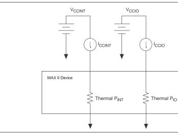
Figure 17–9. Thermal Power Representation
