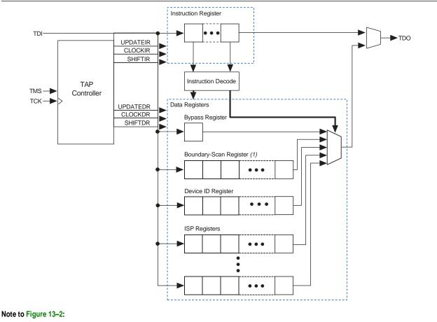
(1) Refer to the JTAG and In-System Programmability chapter in the MAX II Device Handbook for the boundary-scan register length in MAX II devices.
