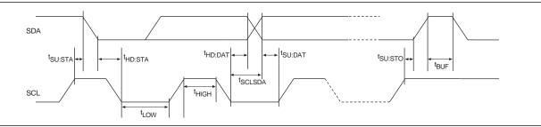
Table 9–6 through Table 9–8 list the timing specification needed for the altufm\_i2c megafunction read/write mode.
