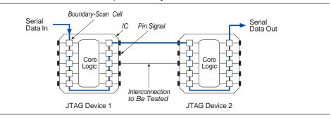
Figure 13-1. IEEE Std. 1149.1 Boundary-Scan Testing
