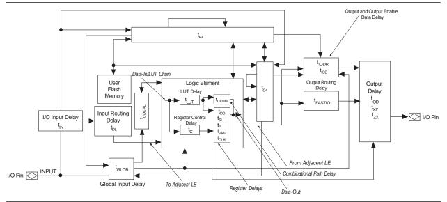
Figure 16-1. MAX II Device Timing Model
