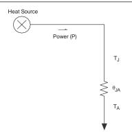
The PowerPlay Early Power Estimator spreadsheet determines the junction-toambient thermal resistance ( $\theta_{JA}$ ) based on the device, package, and airflow selected in the main input parameters.
