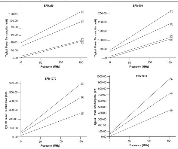
Figure 17–1. Power Consumption versus Frequency for MAX II Devices (Note 1), (2)
