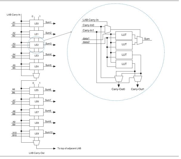
The Quartus II software automatically creates carry chain logic during design processing, or you can create it manually during design entry. Parameterized functions such as LPM functions automatically take advantage of carry chains for the appropriate functions. The Quartus II software creates carry chains longer than 10 LEs by linking adjacent LABs within the same row together automatically. A carry chain can extend horizontally up to one full LAB row, but does not extend between LAB rows.
