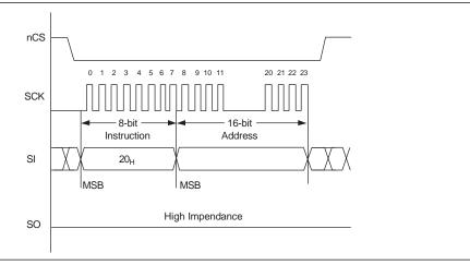
Figure 9-31 shows the SECTOR-ERASE operation sequence for Base mode.
