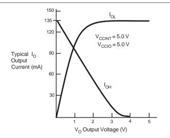
As shown above,  $R_1 = 5.0 \text{ V}/135 \text{ mA}$ .
