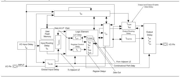
The timing characteristics of any signal path can be derived from the timing model and parameters of a particular device. External timing parameters, which represent pin-to-pin timing delays, can be calculated as the sum of internal parameters.
