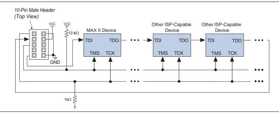
The TMS pin is pulled high so that the TAP controller will remain in the TEST\_LOGIC/RESET state even if there is input from TCK. To prevent TCK from pulsing high, the TCK pin is pulled low during power-up. Pulling TCK high is not recommended because an increase in the power supply to the pull-up resistor causes the TCK to pulse high; thus, it is possible for the TAP controller to reach an unintended state.
