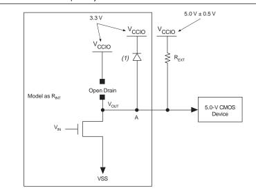
Figure 8-3. MAX II Device Compatibility with 5.0-V CMOS Devices
