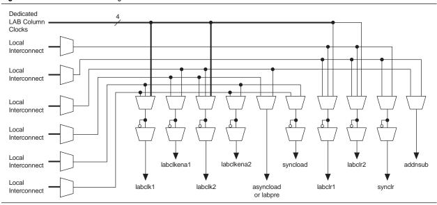
Figure 2–5. LAB-Wide Control Signals
