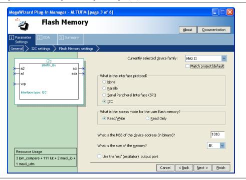
The UFM block's internal oscillator is always running when the altufm\_i2c megafunction is instantiated for both read-only and read/write interfaces.
