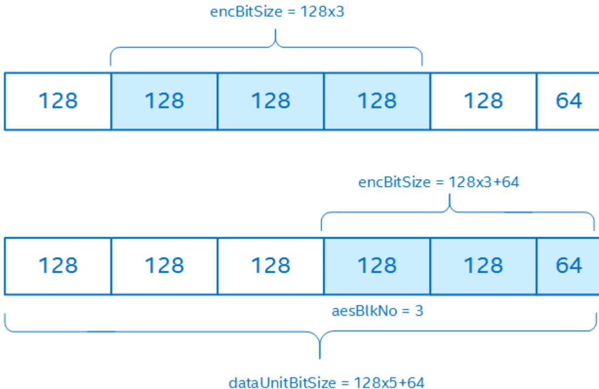
The XTS-AES block cipher uses tweak values to ensure that each data unit is processed differently. A tweak value is a 128-bit integer that represents the logical position of the data unit. The tweak values are assigned to the data units consecutively, starting from an arbitrary non-negative integer. Before calling the function, convert the tweak value into a 16-byte little-endian array. For example, the tweak value 0x123456789A corresponds to the byte array
