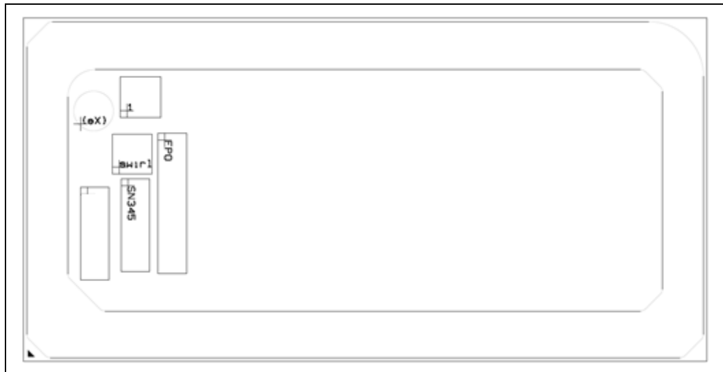
Figure 3. Processor Based on U15 Processor Line Chip Package BGA Top-Side Markings
