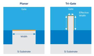
**Figure 1.** Effective Channel Widths of Planar and Tri-Gate Transistor Structures
