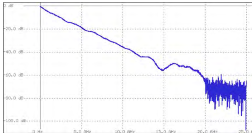
Figure 2. Insertion Loss Plot for 30" Nelco 4000-13 SI Backplane
