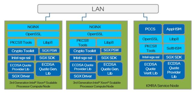
Figure 8: Ansible Deployment of KMRA Components Across Multiple 3<sup>rd</sup> Generation Intel® Xeon® Scalable Processor Compute Nodes and a Service Node
