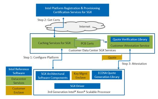
Figure 3: Intel® SGX Data Center Attestation Deployment Architecture
