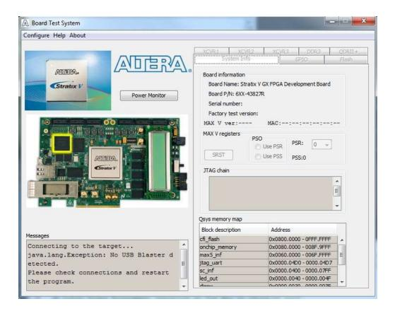
The Board Test System GUI is shown below:
