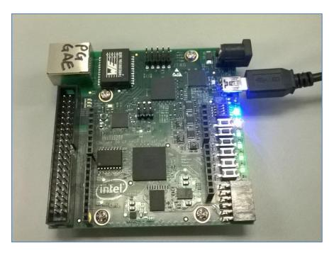
Figure 1. Cyclone 10 LP FPGA Evaluation Kit
