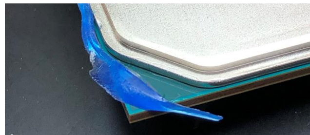
Sealant peel-off after wash process
