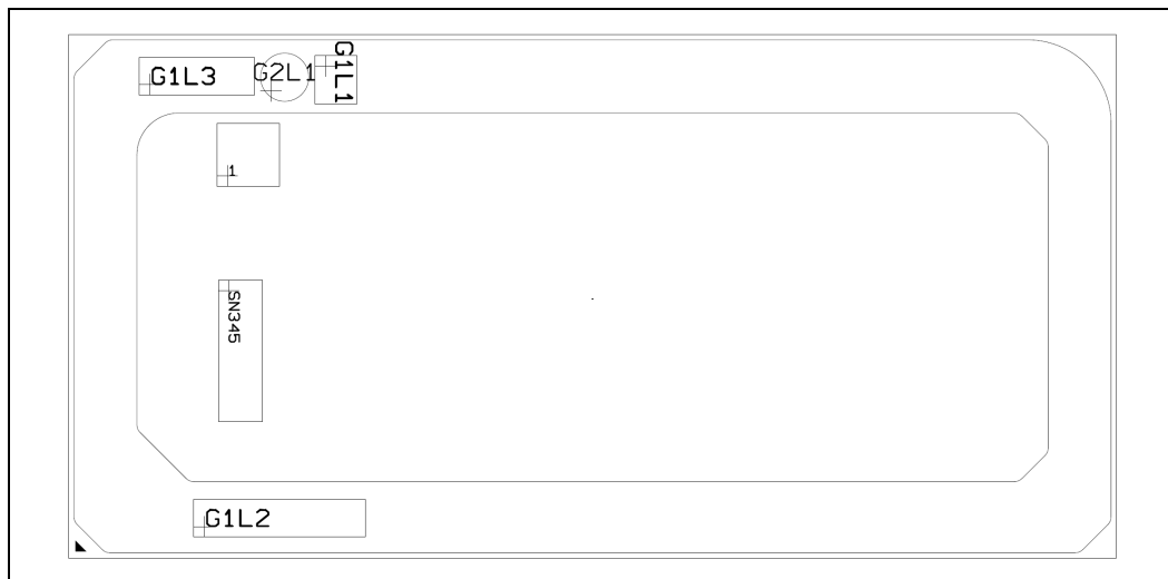
Figure 2-2. Processor Based on H/H-Refresh/P Processor Line Chip Package LGA Top-Side Markings
