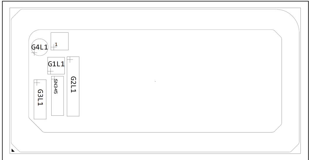
Figure 2-4. Processor Based on U/U-Refresh Processor Line Chip Package LGA Top-Side Markings
