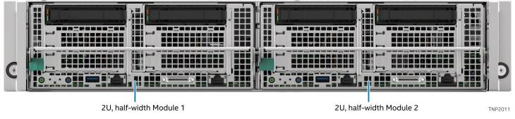
Figure 21. Module Identification for Two-Module System Configuration – Chassis IPCs: FC2HLC21W3, FC2HAC21W3, FC2HAC16W3
