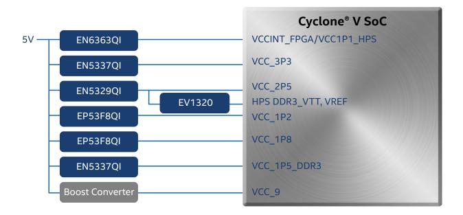
Intel recommends powering the Cyclone® V SoC with Intel® Enpirion® Power Solutions. Here are the recommended power supplies for the Terasic\* DE-10 Nano development board:
