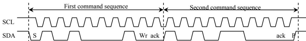
*Please note that the time for the Interrupt Service Routine is not shown here. It is assumed that the ISR is much faster than the I<sup>2</sup>C cycle time, and therefore not visible.*
