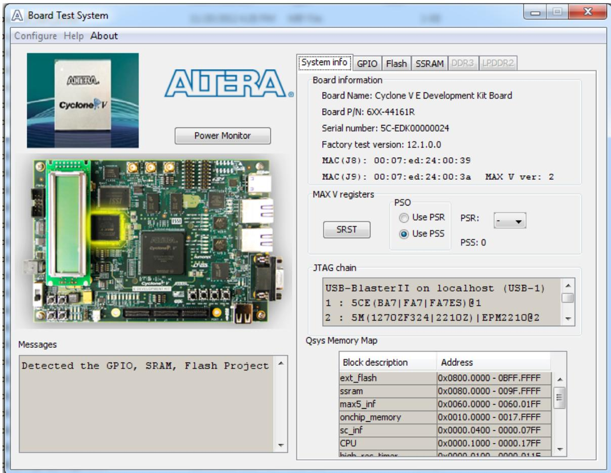
Several designs are provided to test the major board features. Each design provides data for one or more tabs in the application. The Configure menu identifies the appropriate design to download to the FPGA for each tab.
