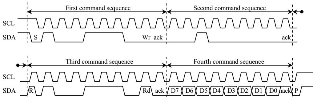
*Please note that the time for the Interrupt Service Routine is not shown here. It is assumed that the ISR is much faster than the I<sup>2</sup>C cycle time, and therefore not visible.*
