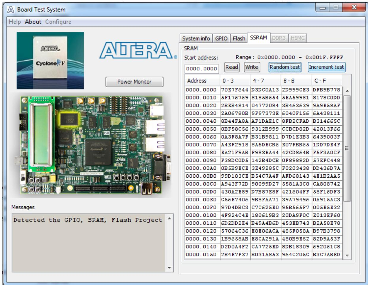
The following sections describe the controls on the **SSRAM** tab.
