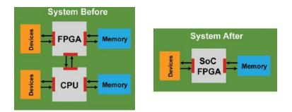
Integrating these technologies on the same piece of silicon eliminates the cost of one of the plastic packages, and saves board space. If both the CPU and FPGA use separate external memories, it may also be possible to consolidate both into one memory device, for further savings.
