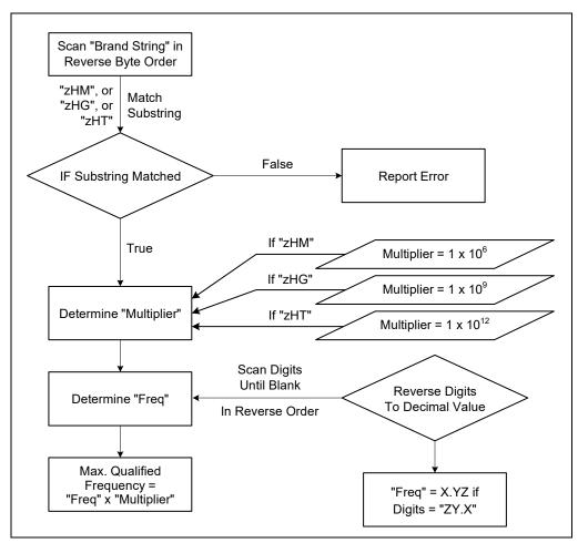
Figure 1-5. Algorithm for Extracting Maximum Processor Frequency
