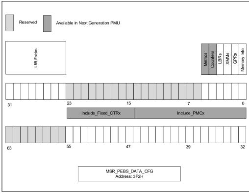
Figure 8-1. Layout of the MSR\_PEBS\_DATA\_CFG Register
