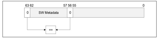
Figure 6-2. Canonicality Check When LAM57 is Enabled for User Pointers with 5-Level Paging
