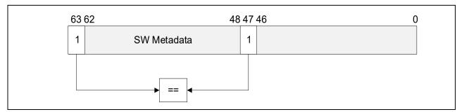
Figure 6-5. Canonicality Check When LAM48 is Enabled for Supervisor Pointers with 4-Level Paging
