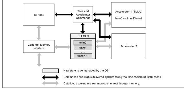
Figure 3-1. Intel® AMX Architecture
