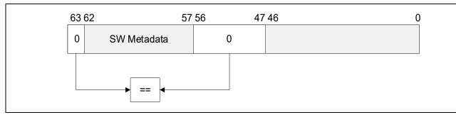
Figure 6-3. Canonicality Check When LAM57 is Enabled for User Pointers with 4-Level Paging
