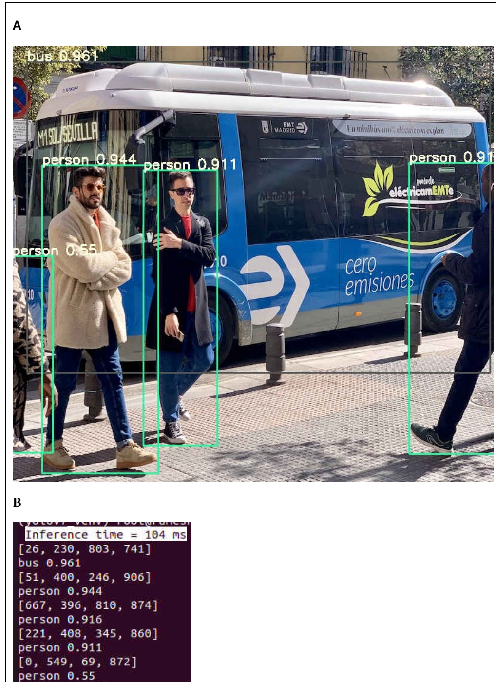
Figure 3. Detection Results of the Optimized YOLOv7 Model with FP32 Precision
