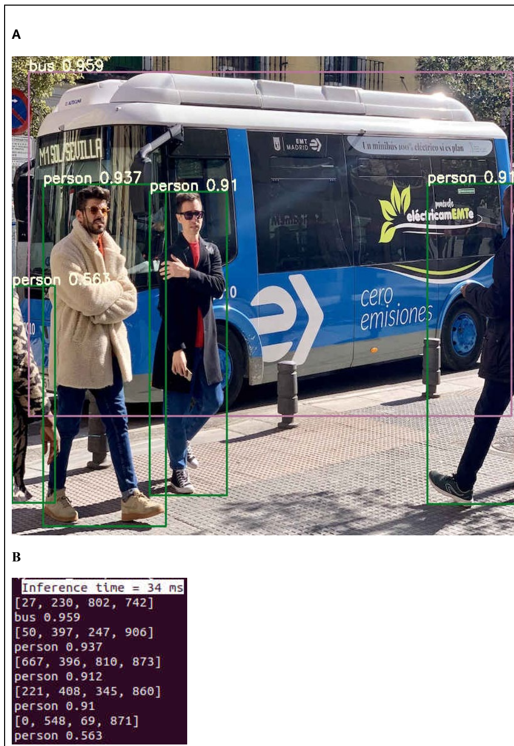
Figure 4. Detection Results of the Quantized YOLOv7 Model with INT8 Precision
