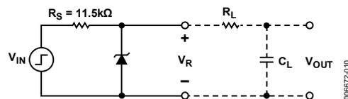
Figure 19. Turn-On, Settling, and Transient Test Circuit
