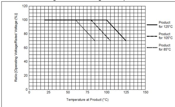
These Part Numbers are designed for use in the circuits where continuous applied voltage to the capacitor is derated than rated voltage, and guarantee Durability Test with 100% x rated voltage as testing voltage at the maximum operating temperature. The voltage and temperature derating conditions on the left are recommended for use to ensure the same reliability level as normal specification.
