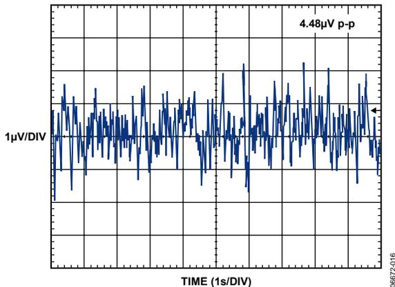
Figure 16. 0.1 Hz to 10 Hz Voltage Noise
