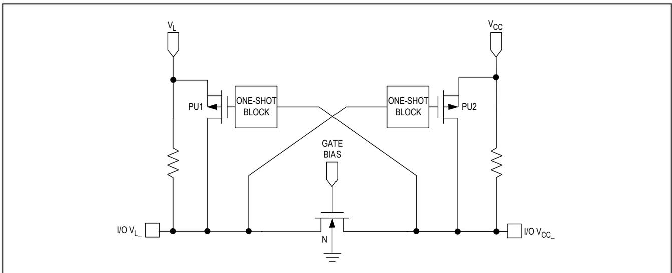
Figure 2b. Functional Diagram, MAX3373E/MAX3378E (1 I/O line)
