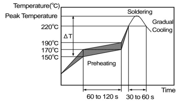
[Allowable Reflow Soldering Temperature and Time]
