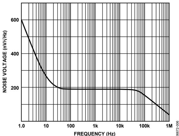
Figure 6. Noise Spectral Density
