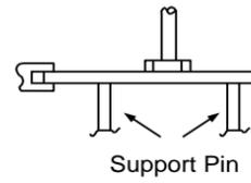
2. Dirt particles and dust accumulated in the suction nozzle and suction mechanism prevent the nozzle from moving smoothly. This creates excessive force on the capacitor during mounting, causing cracked chips. Also, the locating claw, when worn out, imposes uneven forces on the chip when positioning, causing cracked chips. The suction nozzle and the locating claw must be maintained, checked and replaced periodically.
