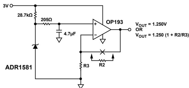
Figure 23. Micropower Buffered Reference
