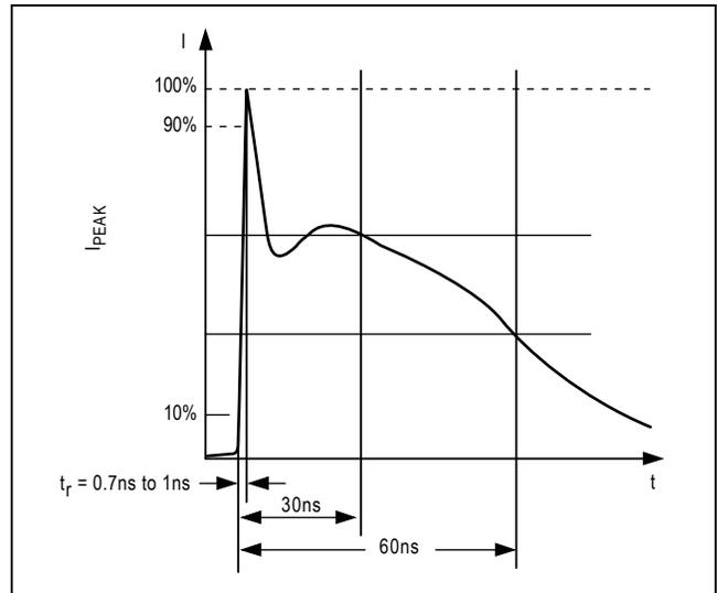
Figure 4b. IEC 1000-4-2 ESD Generator Current Waveform
