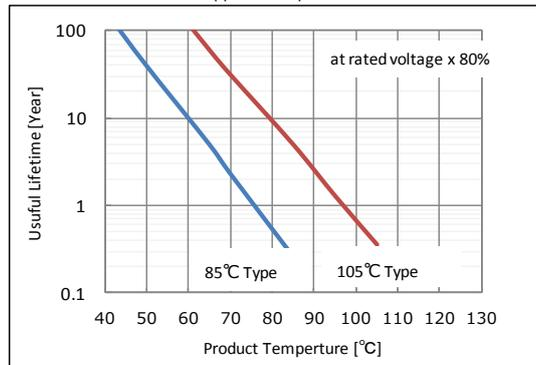
These MLCC products are designed for use in devices with a typical lifetime of less than 5 years. (Examples: Cellular phone, Smartphone, Tablet PC, Digital camera, Watch, Electronics dictionary, Small-scale server, IPC-9592B class1 equipment, etc.) These MLCC products are designed so that the useful lifetime can be extended longer than 5 years under the following conditions:
