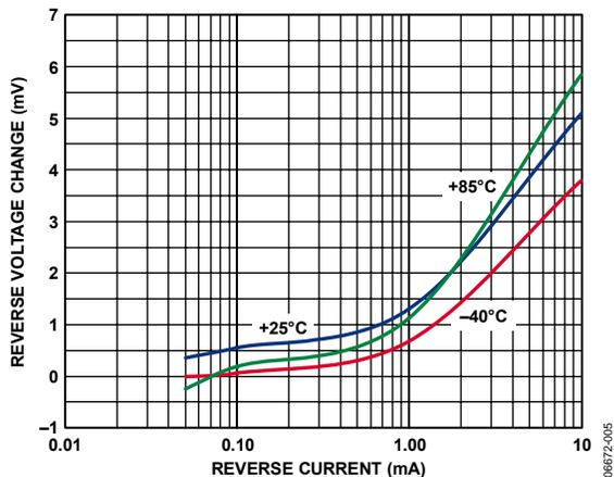
Figure 5. Output Voltage Error vs. Reverse Current
