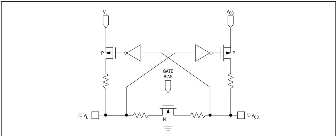
Figure 2a. Functional Diagram, MAX3372E/MAX3377E (1 I/O line)
