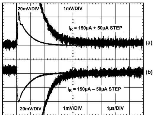
Figure 21. Transient Settling
