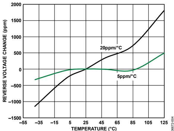
Figure 4. Output Drift for Different Temperature Characteristics
