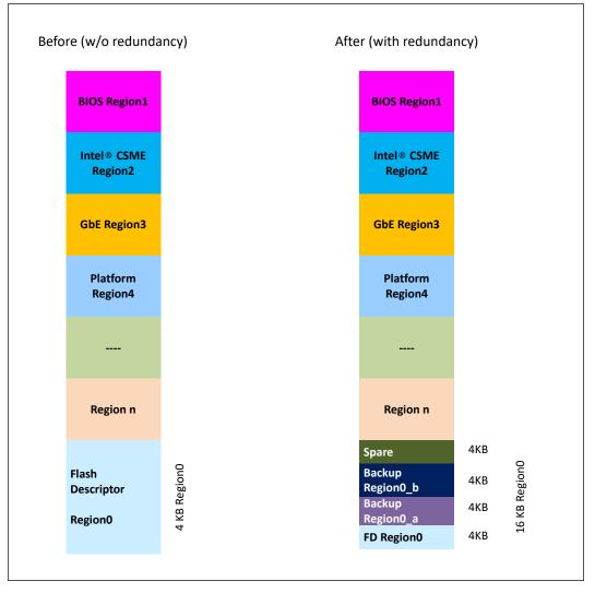
In the main and backup descriptor regions, the following fields are defined for the descriptor integrity check and recovery. Before SPI controller reads the descriptor, it
