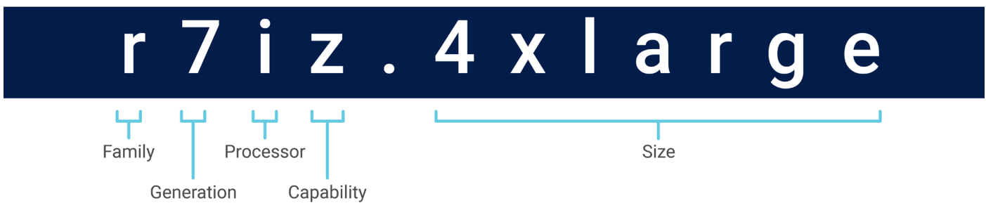
Figure 1 | Amazon EC2® instances follow an architectural naming system that can help you choose the right cloud instance for your needs
