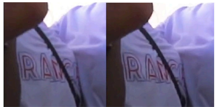
Figure 4. Side by side view of the output of Lanczos (left) and Enhanced RAISR (right) upscale of a T-shirt.
