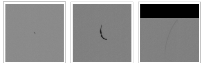
Figure 3. Types of wafer defects detected by the inline vision inspection system.
