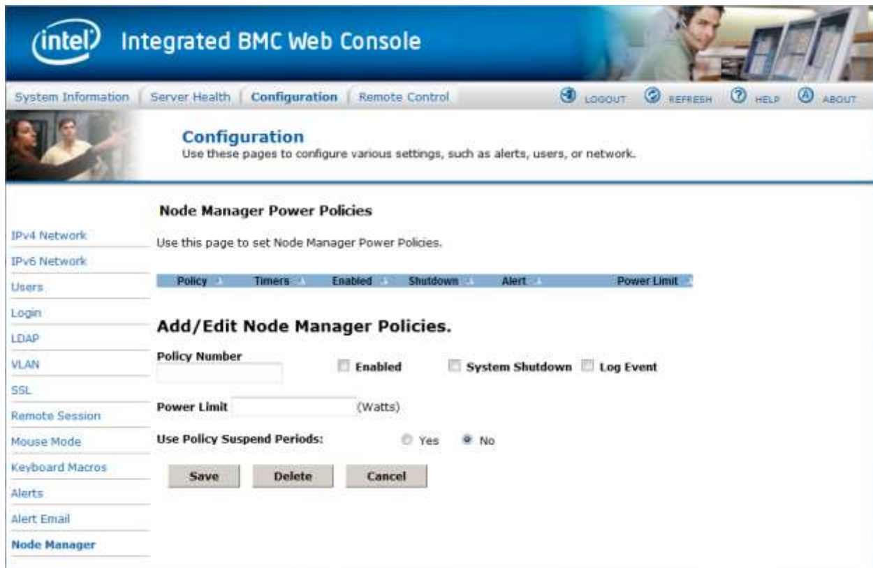
Figure 101: Configuration Node Manager Page on Intel® Server Boards and Systems Based on Intel® Xeon® Processor E5-4600/2600/2400/1600/1400 (v1&v2) Product Families, S1200V3RP and Intel® Server Boards and Systems Based on Intel® Xeon® Processor E5-2600 V3 --- S2600WT, S2600KP, S2600TP and S2600CW
