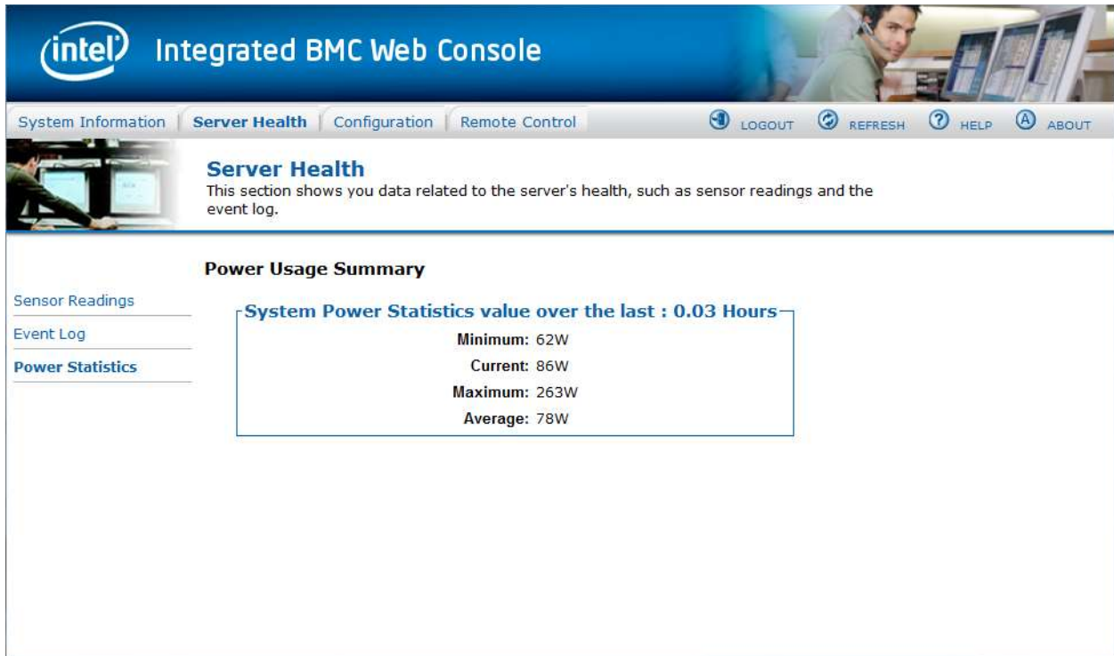
Figure 77: Server Health Power Statistic Page on Intel® Server Boards and Systems Based on Intel® Xeon® Processor E5-4600/2600/2400/1600/1400 (v1&v2) Product Families
