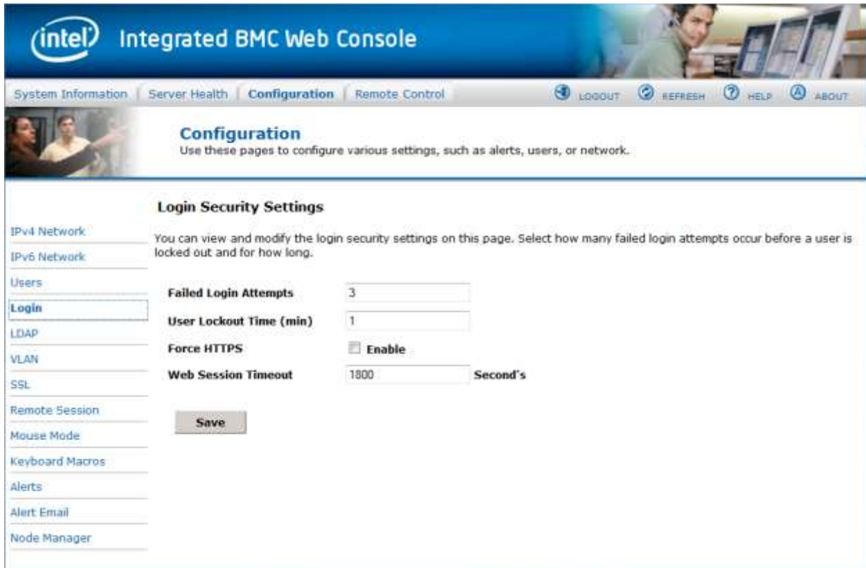
Figure 85: Configuration Login Security Settings Page on Intel® Server Boards and Systems Based on Intel® Xeon® Processor E5-4600/2600/2400/1600/1400 (v1&v2) Product Families, S1200V3RP Product Family and Intel® Server Boards and Systems Based on Intel® Xeon® Processor E5-2600 V3 --- S2600WT, S2600KP, S2600TP and S2600CW
