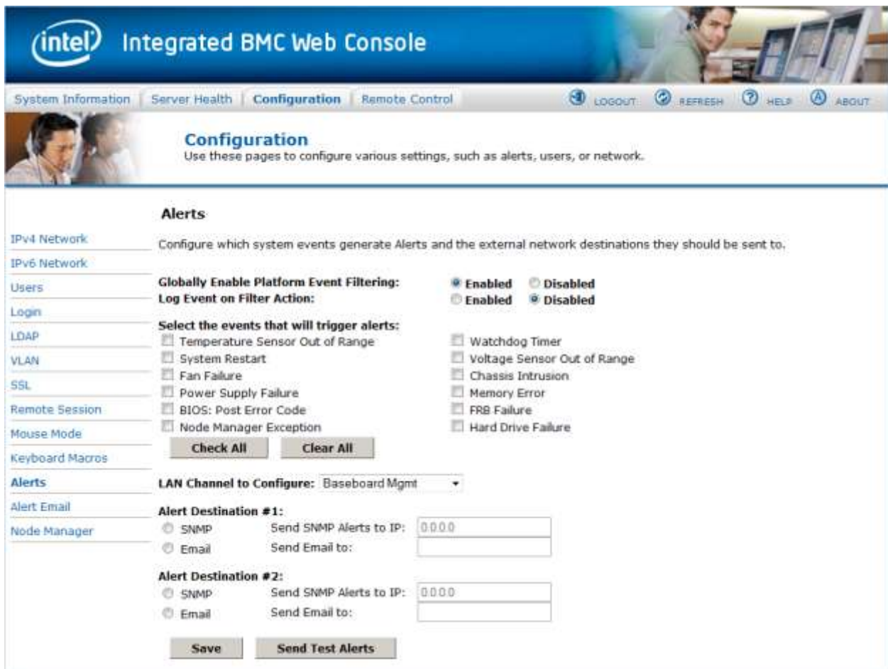
Figure 99: Configuration Alerts Page on Intel® Server Boards and Systems Based on Intel® Xeon® Processor E5-4600/2600/2400/1600/1400 (v1&v2) Product Families, S1200V3RP and Intel® Server Boards and Systems Based on Intel® Xeon® Processor E5-2600 V3 --- S2600WT, S2600KP, S2600TP and S2600CW
