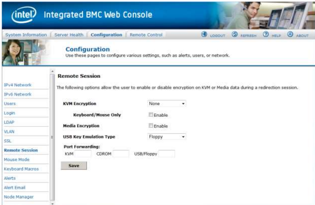
Figure 90: Configuration Remote Session Page on Intel® Server Boards and Systems Based on Intel® Xeon® Processor E5-4600/2600/2400/1600/1400 (v1&v2) Product Families
