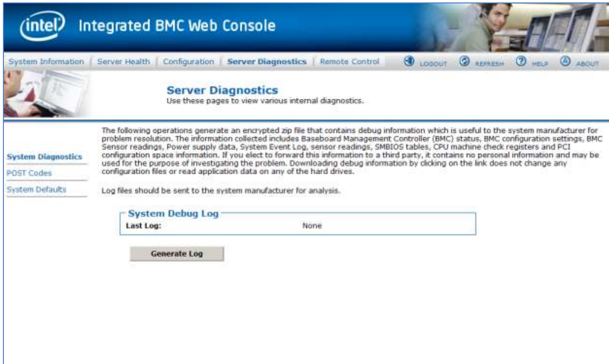
Figure 67: System Information System Debug Log Page on Intel® Server Boards and Systems Based on Intel® Xeon® Processor E5-2600 V3 --- S2600WT, S2600KP, S2600TP and S2600CW
