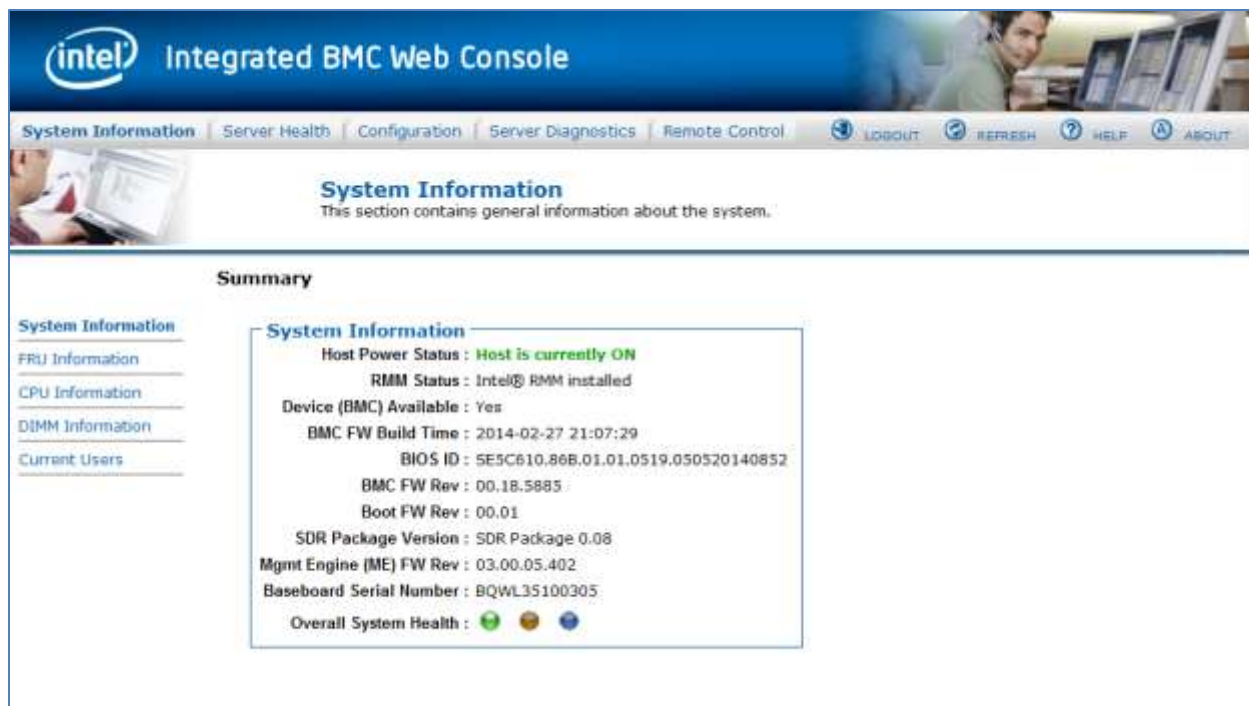
Figure 63: System Information Page on Intel® Server Boards and Systems Based on Intel® Xeon® Processor E5-2600 V3 --- S2600WT, S2600KP, S2600TP and S2600CW
