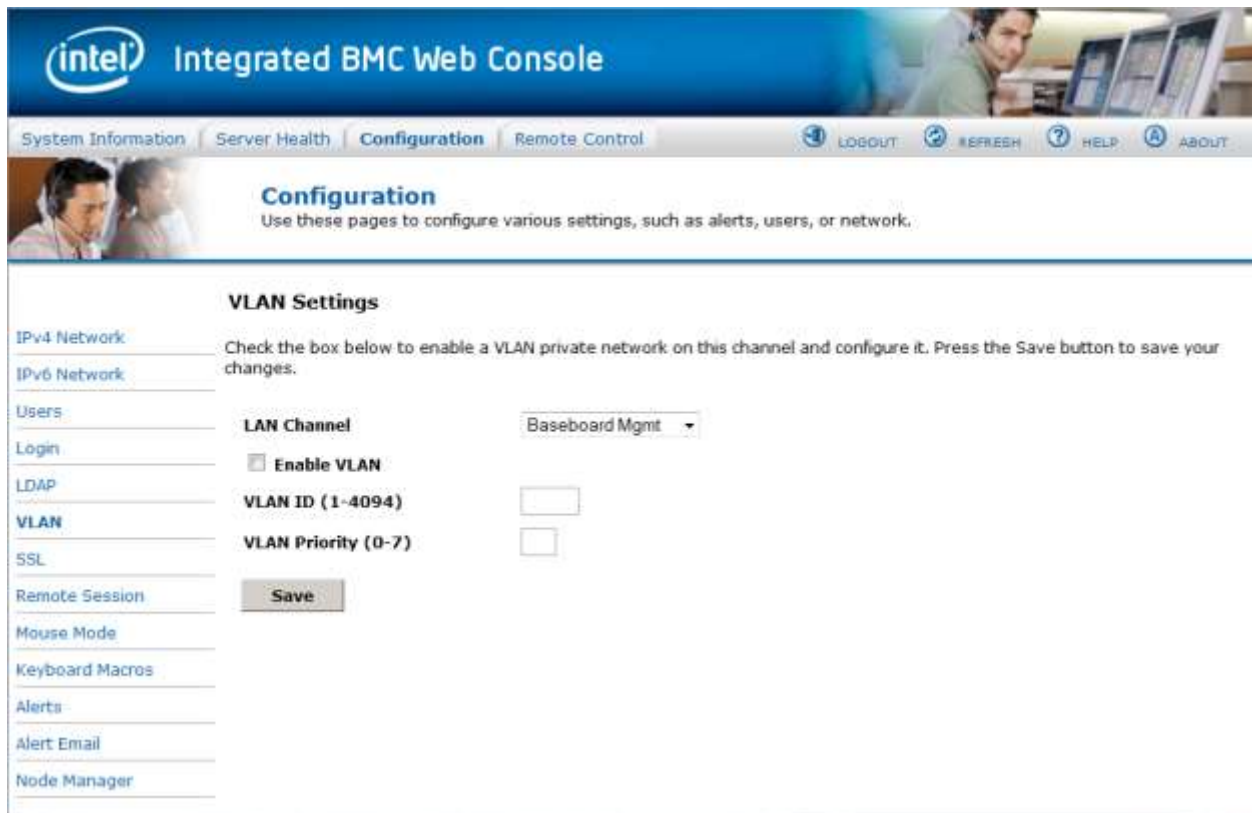
Figure 87: Configuration VLAN Settings on Intel® Server Boards and Systems Based on Intel® Xeon® Processor E5-4600/2600/2400/1600/1400 (v1&v2) Product Families, S1200V3RP and Intel® Server Boards and Systems Based on Intel® Xeon® Processor E5-2600 V3 --- S2600WT, S2600KP, S2600TP and S2600CW Product Family
