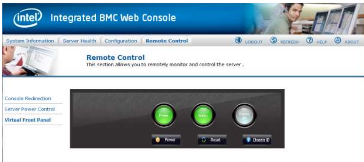
Figure 107: Remote Control Virtual Front Panel Page on Intel® Server Boards and Systems Based on Intel® Xeon® Processor E5-4600/2600/2400/1600/1400 (v1&v2) Product Families, S1200V3RP and Intel® Server Boards and Systems Based on Intel® Xeon® Processor E5-2600 V3 --- S2600WT, S2600KP, S2600TP and S2600CW
