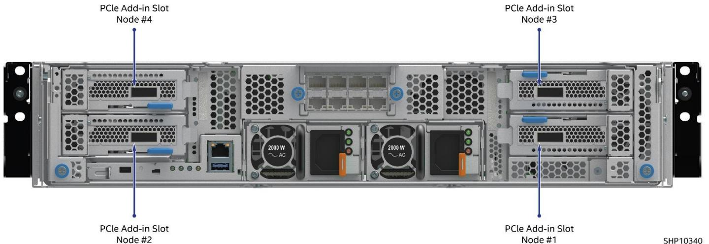
**Figure 56. PCIe\* Add-in Card location, system rear**
