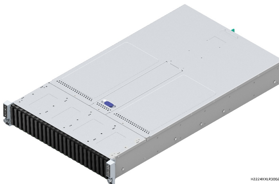
Figure 2. Server chassis overview – 24 x 2.5" drive bay
