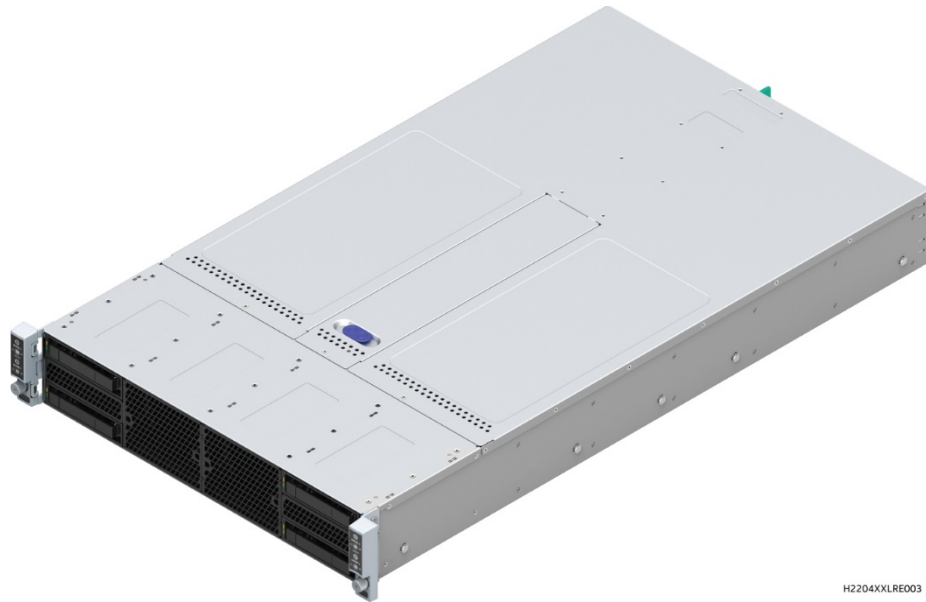
Figure 3. Server chassis overview – 4 x 3.5" drive bay
